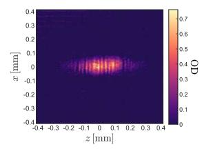
Figure 1: Interference fringes from two separate BECs expanding into each other in our apparatus. The BECs are formed in a double-well, then allowed to evolve in a cigar shaped trap.
